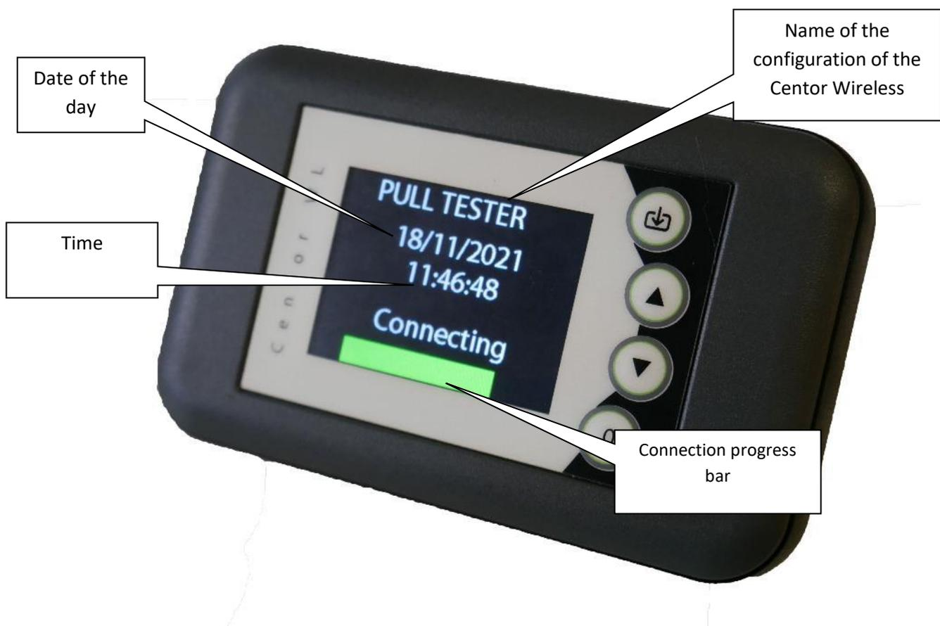
If you have already connected a sensor and it is turned on, Centor Wireless will automatically connect to it and you will be taken to the measurement screen. Otherwise, Centor Wireless will search for available sensors.
