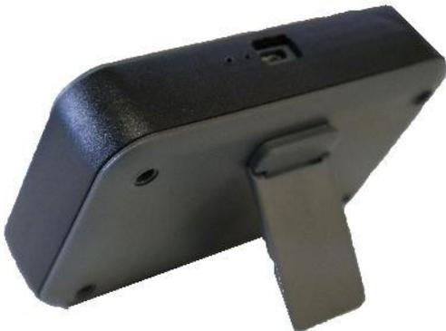
Adjustable foot attached to the back of the case
