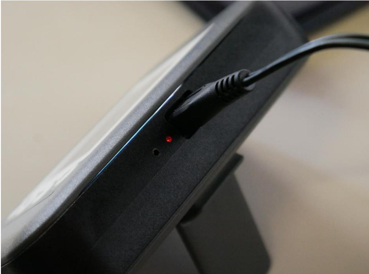
Plug the supplied charger into the USB port to charge the Centor Wireless display. The red LED lights up during charging and goes out once the battery is charged.
